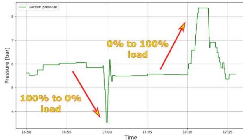
Figure 10. Low pressure compressor reaction to sudden load change.
