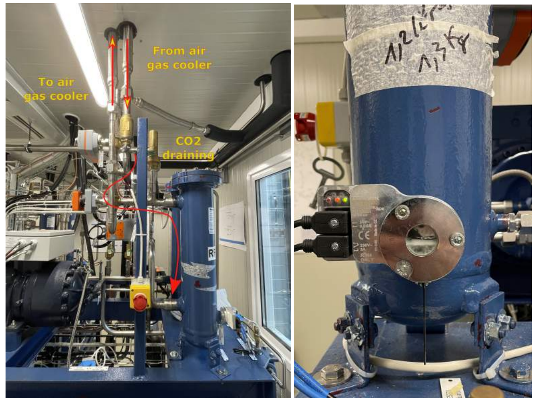
Figure 11. (left) Path followed by CO 2 being draining into separators. (right) Visualisation through oil level sensor sight glass of CO 2 condensing inside oil separator.
